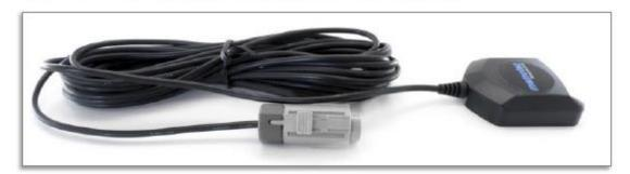
To guarantee a quick change of the memorykey during a pit stop it must be reached easily. Therefore the extension cable (connected to the logger) has to be placed on the passenger side.
