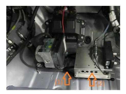
2. Fix the boost pressure sensor on the base. Connect the Teflon pipe from the boost sensor to the inlet manifold. Pass the pipe through the engine bay wall. Following the fuel pipe is an option, but you can find other ways.
